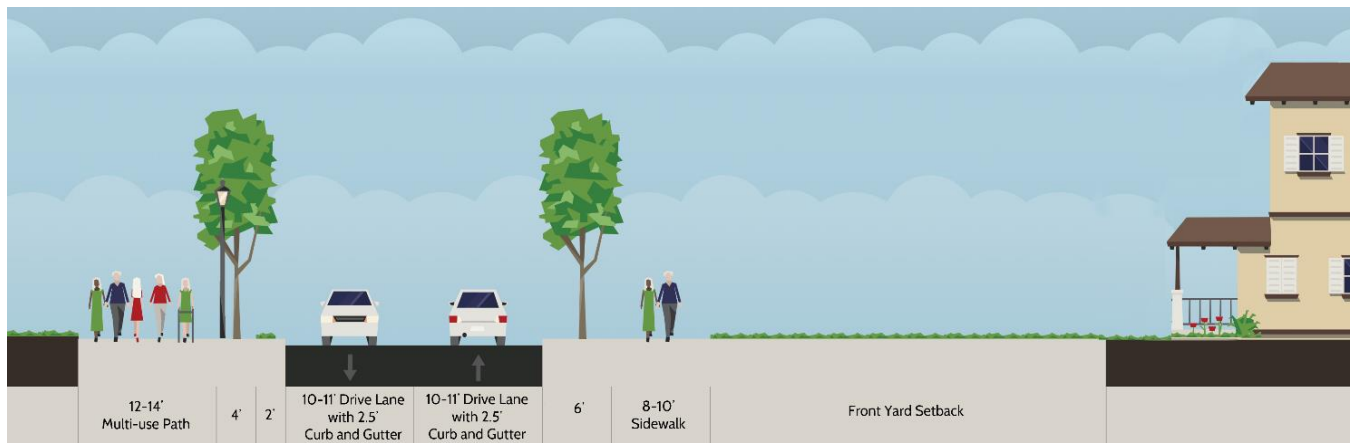
Figure 17 Typical Section for Collector Road in Residential Area with Multiuse Path
